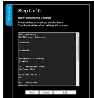
The NetComm Wireless Router will attempt to connect using the details you have entered. This can take up to **2 minutes**. When a connection is successfully made, the Internet Connection LED on the front of the unit illuminates.
